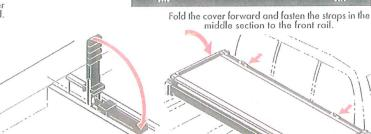
IMPORTANT: Before folding the second section of the cover, rear clamps must be stowed securely into rail.
