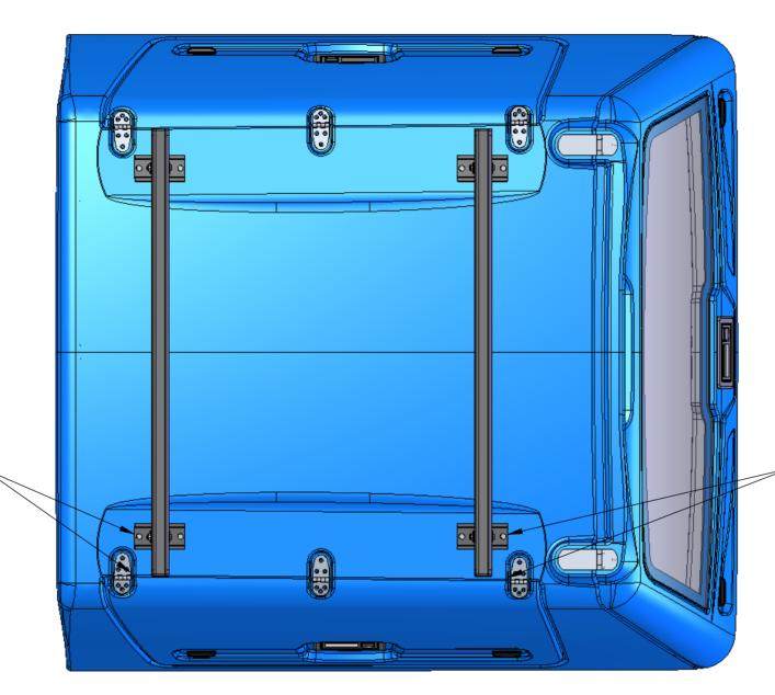
Foten placeras i linje med gångjärnets framkant The foot is placed in line with the hinge
