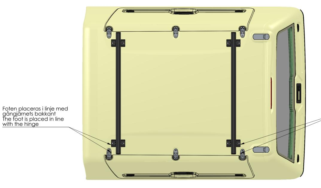
Foten placeras i linje med gångjärnets framkant The foot is placed in line with the hinge
