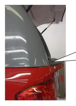
Mount hardtop lower-rear corner aligned with the cargo bed rear corner.
