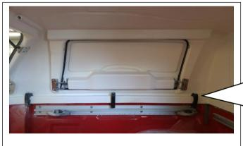
Center the cover sideways on the load bin and place the clamps acc. to the image. Pull the cover towards the edge of the bin with clamps
