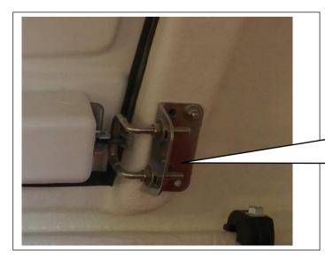
Check that the doors close easily and that the lock is correctly adjusted, if necessary adjust the lock or locking strap.
