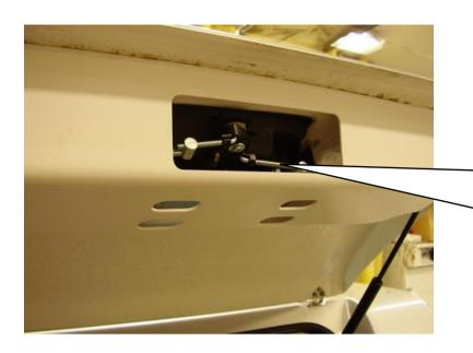
It is possible to adjust the length of the locking rods by loosening the plastic clip and turning the locking rod which is screwed into the joint against the locking hook.
